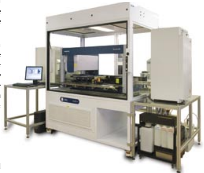
Figure 1: Fully automated cell culture system based on the MICROLAB® STAR platform. The system is housed in a laminar flow hood and serves two external Kendro incubators (4°C/37°C).
